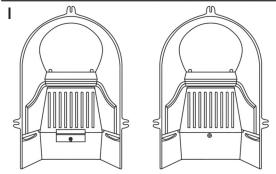
Remove the Firebrick Retaining Plate by removing the  $1 \times M6$  Bolt, Washer and Nut.
