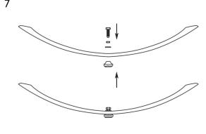
Attach the Ashpan Handle to the Ashpan using Ix M6 Bolt, Ix M6 Washer and Ix M6 Nut.
