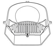
Lay Fireplace Back down on level ground. Position Firebrick in place and then insert I  $\times$  M6 Bolt, passing through Washer and Nut, into the hole just below the Firebrick. Insert Grate into the groves on the Fireplace Back, passing the fixing lug over the M6 Bolt. Secure in place by tightening Bolt.
