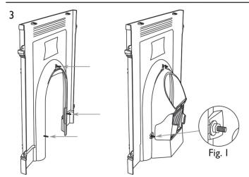
Insert the 3 M6 Studs into the back of the Fireplace Fascia. Attach Fireplace Back to the back of the Fireplace Fascia, ensuring that the M6 Studs pass through the fixing brackets on the Fireplace Back. Secure and tighten using 3 M6 Washers and 3 M6 Nuts, as Fig. I.
